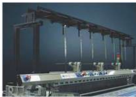
可配置绞织机构，绞织与正常平行织造转换便捷，实现一机多用。 LENO weaving mechanism can be configured. Easy conversion between LENO weaving and normal parallel weaving ; to achieve a multi-purpose machine.
