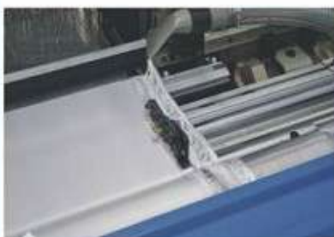
采用砍刀式纬剪边剪 Chopper type weft cutter and Selvage cutter
