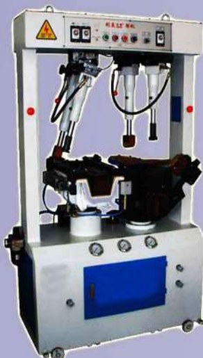
SL-LZ690 Universal hydraulic sole attaching machine
