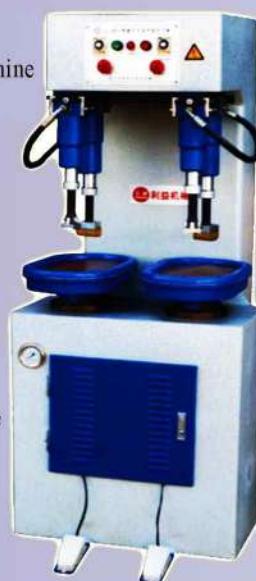
SL-LZ609 Double head hydraulic sole attaching machine
