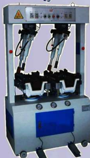
SL-LZ670 Travelling head wall type sole attaching machine
