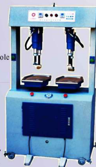
SL-LZXDY-2 Double head cover type sole attaching machine
