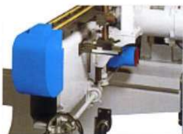
Thickness of cut at both ends can be set as desired.
