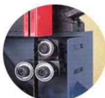
Lower ball bearing blade guide system
