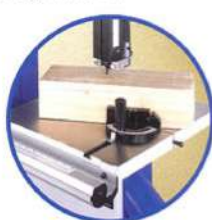
Miter gauge for various angle cutting (optional)
