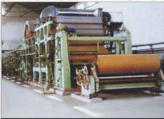
Double-dryer and double cylinder mould corrugated paper production line
