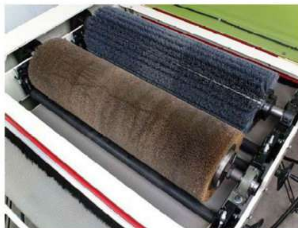
Two rollers 1st : steel brush 2nd : abrasive nylon brush
