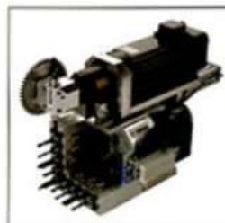
9 Vertical Boring and 1 Saw Combination Head
