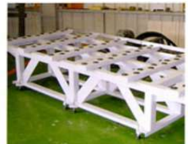
ROLLER CONVEYOR TABLES IN FRONT AND BACK OF MACHINE AND FLOATING TABLE TOP SYSTEM ◆ This can eliminate downtime for parts changing and also full board sheets can move more easily.
