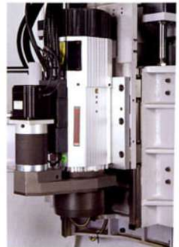
C-Axis Rotation Mechanism ◆ May process any angle between 0° ~ 360° for side processing and saw cutting.
