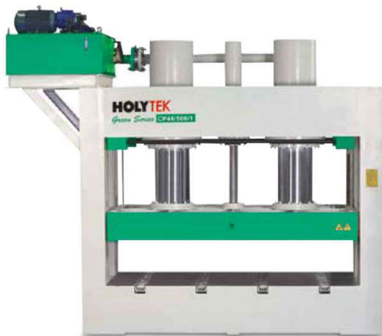
CP48/100/1 Hydraulic Cold Press (with roller device)
