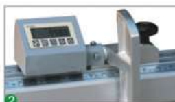
2 Digital display on the transverse guiding ruler
