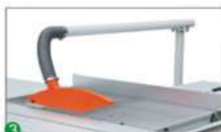
3 Simple dust sucking device
