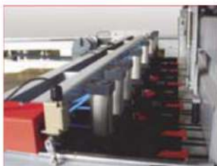
*Floating Clamps -Designed for reducing panel scratching to a minimum.
