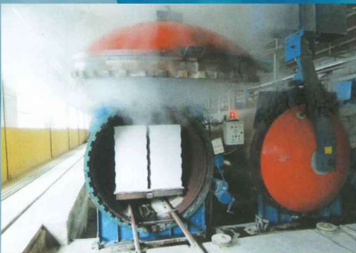
FINISHED BLOCK OUT OF AUTOCLAVE
