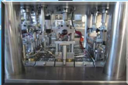
4. Auto charing sealing film , The photoelectric tracking device can be assure of the seal design correct.
