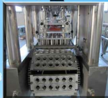
5. 2 times auto sealing unit , and auto cutting unit
