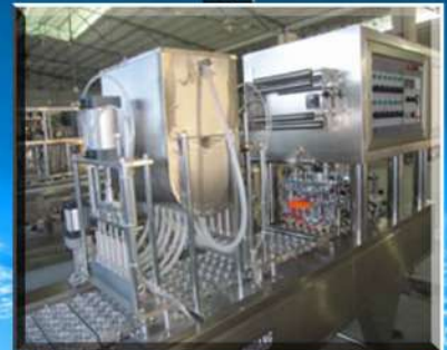
3. 2 times auto filling unit, filling hopper with liquid level controlerco Auto Filler
