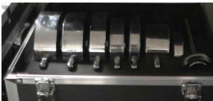
Eight level removable weight (0.325 till 21.6 kg)
