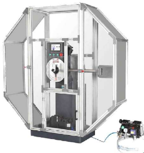
PIT452G with multi-purpose fixture for Charpy & Izod test
